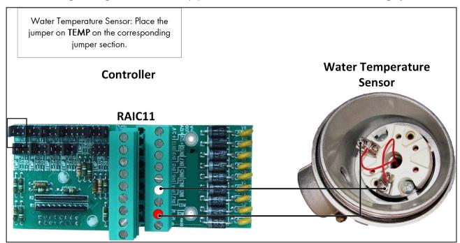
Connect the sensor to an input port and a COM port.
