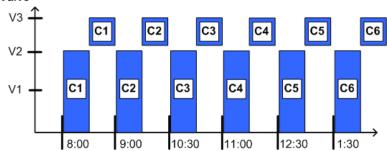
Valve 1 & 2 run six cycles simultaneously on Run Time & Dosing Program 1, Valve 3 runs after Valves 1 & 2 on Run Time & Dosing Program 2, with different/interchangeable start times.
