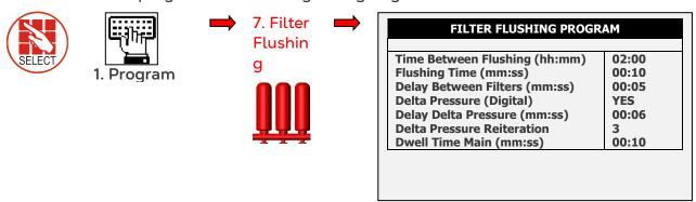
NOTE Filter flush process can start only after main water line is full. The default time is one minute; see Menu 3.3.
