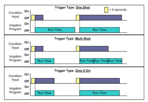
Green Field ECO supports up to 15 extension programs defining which trigger initiates irrigation. In each program, the start and stop trigger must be the same type (meaning both must be dry contact or analog sensor).
