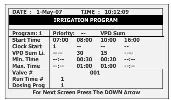
Irrigation based on VPD Sum can take place only during the VPD time frame. Refer to 6.1 SETUP > TIME & DATE to define the start and end time for VPD Sum. Normally, this parameter is defined during installation.
