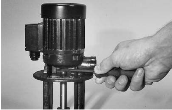
Figure 5.1 Checking the direction of rotation
