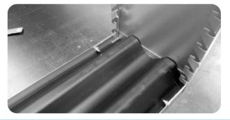
Start to mount the plastic waves: insert the first wave under the first tooth.
