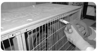
To install the hook, cut from the fan the safety mesh with a diagonal pliers but do not remove the safety protection for motor in order to comply with safety requirement.
