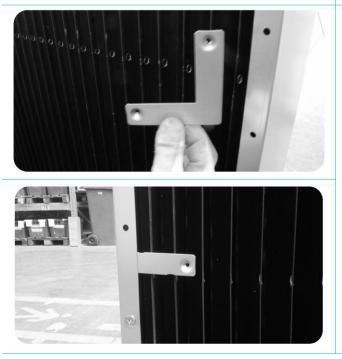
Insert qty. 4 angle brackets and fix them by means of qty. 4 self-tapping screws (flat head - 6.3x16).
