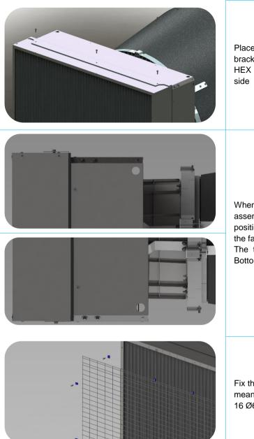
Place the filter between the two brackets by means of 3 M08×25 HEX SCREWS w/flange for each side
