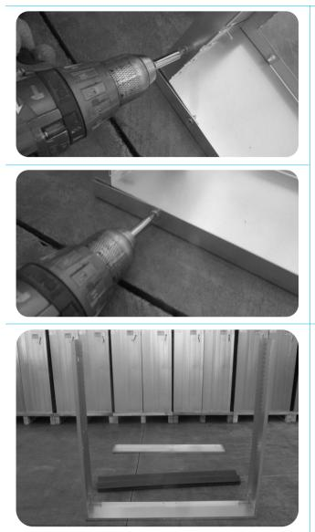
Assemble the top panel - same shape as bottom panel but without holes - together with the free side of the side panel by means of qty. 2 self-tapping screw (round head - 6.3x19), qty. 2 angle brackets and qty. 4 self-tapping screws (flat head -6.3x16).
