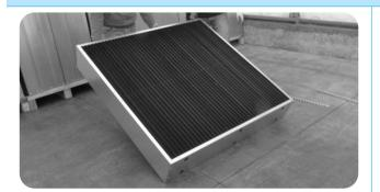
Turn the filter 90° to gain the operating position. The bottom panel should adhere to the floor.
