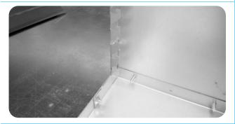
Assemble the bottom panel (the one with 3 holes in the middle) together with the side panel by means of qty. 2 self-tapping screw (round head - 6.3x19), qty. 2 angle brackets and qty. 4 self-tapping screws (flat head - 6.3x16).
