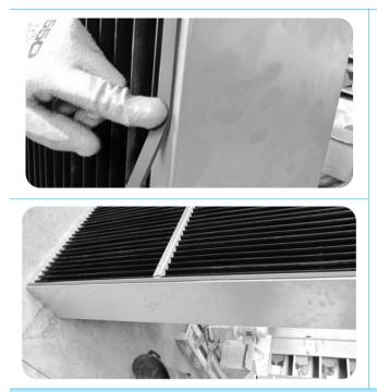
Apply the EPDM strip on the 2 lateral panels and on the bottom panel of the Light Filter.
