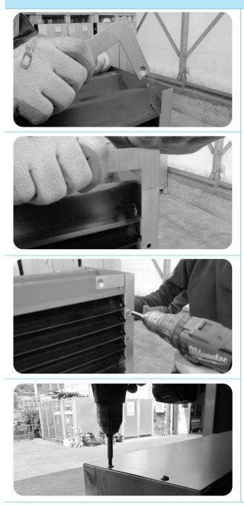
Assemble the angle brackets on the 2 panels (top and bottom) and insert the side panel. Fix them by means of qty. 8 selftapping screws (flat head -6.3x16) to the angle brackets plus 2 screws (round head -6.3x19), one for each panel.
