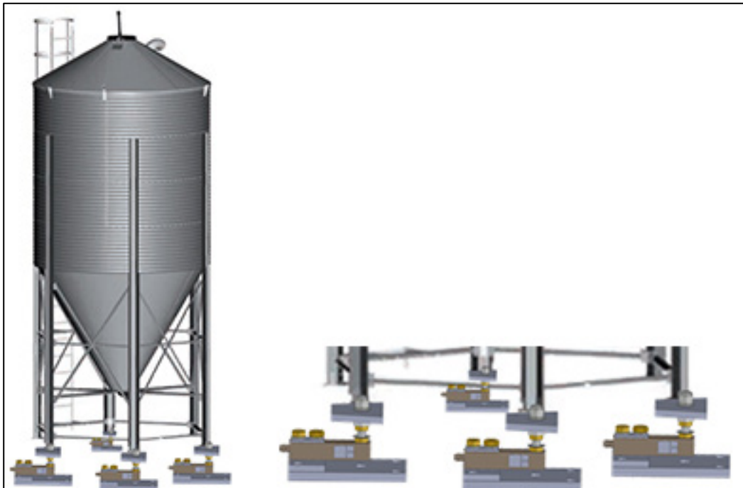
Figure 8: Silo Legs and Load Cells
