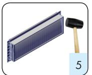
Properly secure the MWI lateral supports using a rubber mallet. Use caution!
