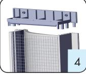
Slide the metal grid in the headers slot.
