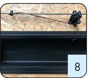
Pass the string through the hole in the curved louver then through the pulley, towards the direction of pulling force. Fix the string to the main pull cable or rod using clamp.
