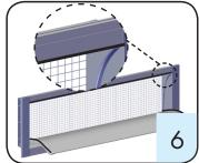
Insert the rubber seal in the top header slot and along door sides.
