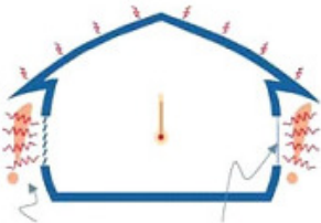
High heat loss through closed fans.
