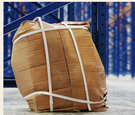
Water damage to stored goods.
