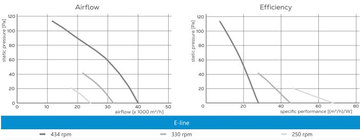
Airflow and efficiency tested in the Munters test chamber in accordance with ANSI/AMCA 210/15 Standard, certified by BESS Lab.
