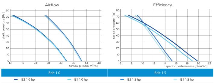
Airflow and efficiency tested in the Munters test chamber in accordance with ANSI/AMCA 210/15 Standard, certified by BESS Lab. \*1 cfm/W = 1.7 (m<sup>3</sup>/h)/W
