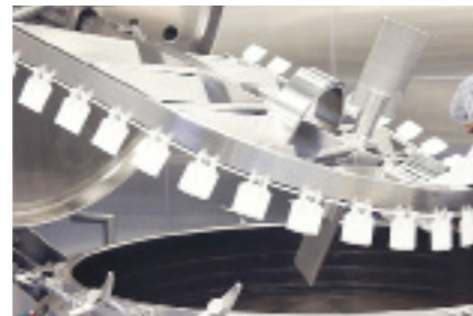
4. Weighing/Mixing/Granulating Optimal environmental conditions ensure that excipients and APIs can be continuously and reliably blended, while avoiding the influence of excess moisture that may affect mechanical and chemical properties. The right balance of moisture ensures that the granulating mixture remains in equilibrium with the air around it, maintaining the required moisture content for granules to form.
