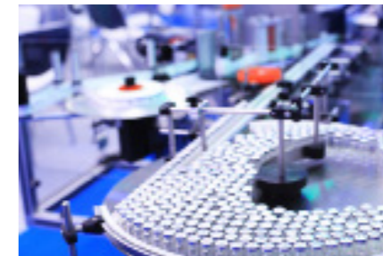
7. Biologics, vaccines, and parenteral products Product quality relies on a clean, controlled manufacturing area. The presence of excessive humidity (>70% Relative Humidity (RH)) increases the potential for microbial growth. Humidity control also reduces drying time after cleaning operations.
