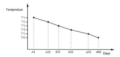
A curve is defined using six points. Each point specifies a day number and a set point for that day. Once the points of the curve are defined, the curve must be activated. The controller will change the temperature set point every hour in a linear fashion between consecutive points of the curve. When the last point of the curve is reached, the temperature set point for that day is maintained until the curve is reactivated.
