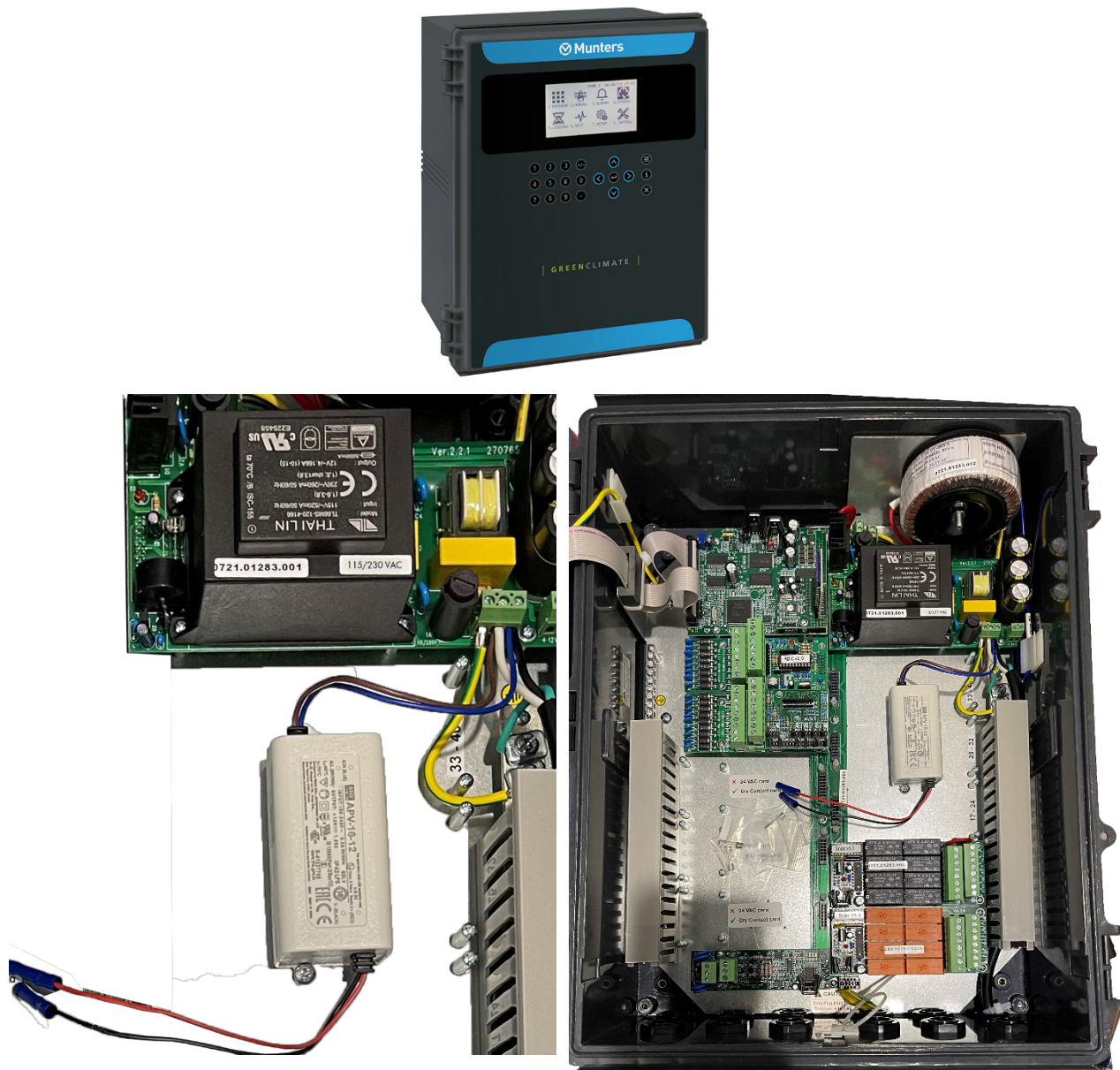
Figure 11: Wiring the CO2 Sensor Power Supply
