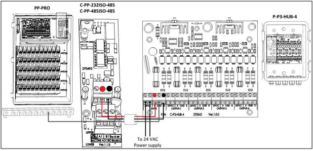
Figure 2: Platinum Pro – HUB Wiring
