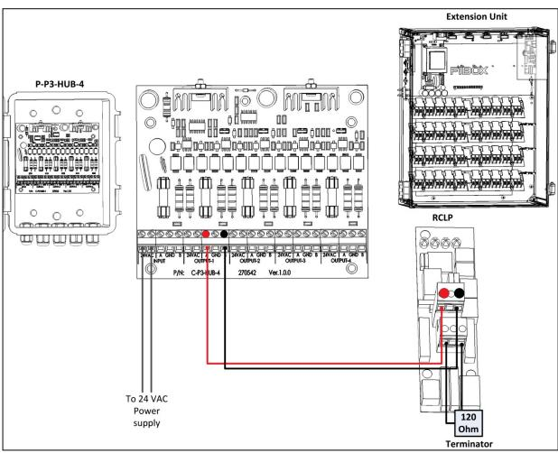
Figure 5: HUB - Platinum Pro Extension Wiring
