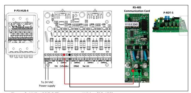
Figure 6: HUB – RDT-5 Thermometer Wiring (RS-485)
