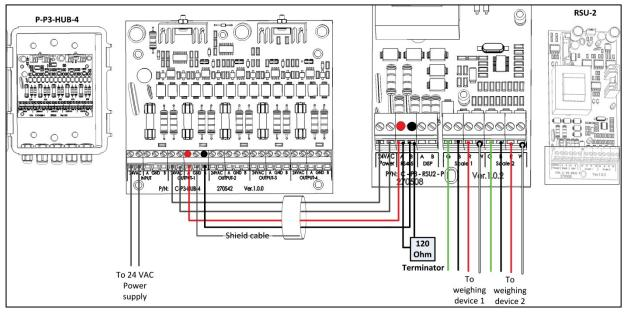
Figure 3: HUB - RSU-2 Pro Wiring
