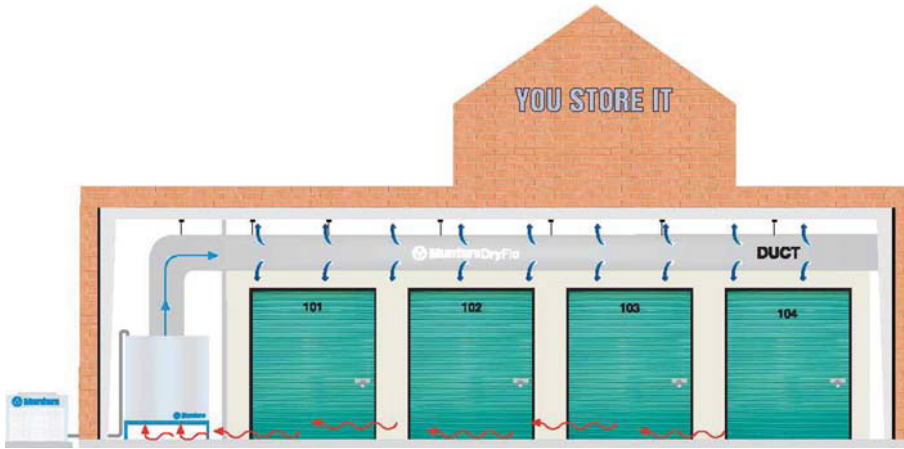
5 Ton DryCool Split System Illustration
