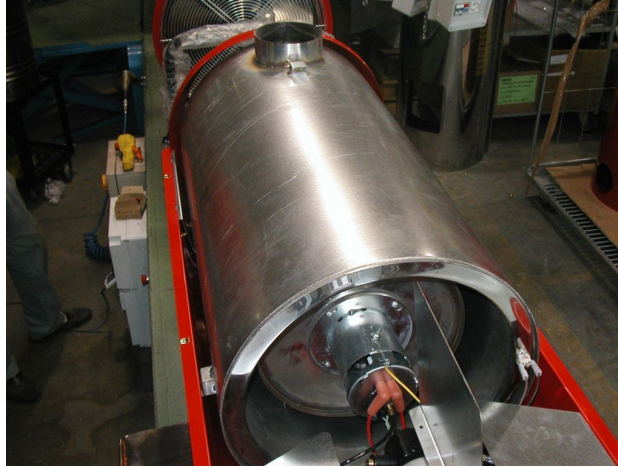
Combustion chamber (MIR)
