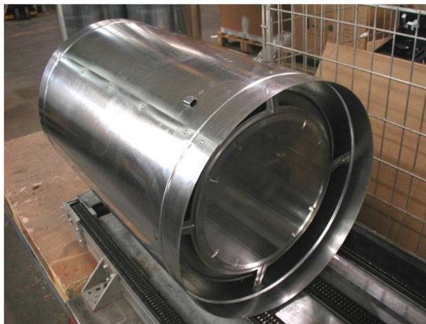
TOR Combustion Chamber
