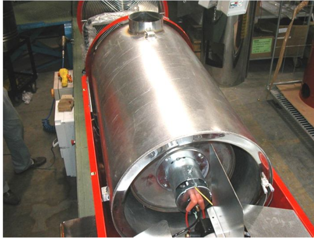
Combustion chamber (MIR)
