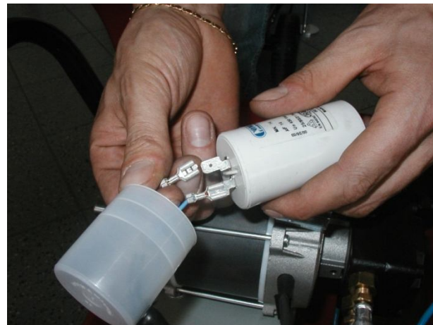
Replacing capacitor Warning! Capacitors may hold an electrical charge and cause electrical shocks.
