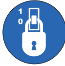
Figure 6.2 Lock against reconnection
